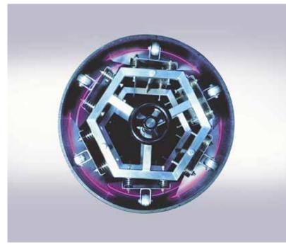
The PipeTEC is designed for treatment of the inside surface of jacket pipes for optimized adhesion of PUR foam which is needed for insulation of the pipe core. The PipeTEC is fully integrated into an extrusion line and ensures a very high level of surface treatment of the entire inside surface.
