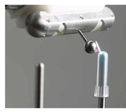
LeakTEC is a powerful electronic tool for non-destructive leak detection of non-conductive single layer materials. The LeakTEC measures a leak between a high-voltage electrode (DC) and counter electrode which can either be grounded or running opposed polarity. The LeakTEC ensures full process control and traceability.
